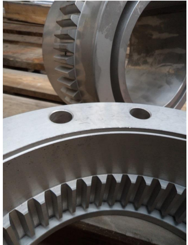
FIG. 15 GEAR HUBS AND SLEEVES IN 42CrMo4 GAS NITRIDED
