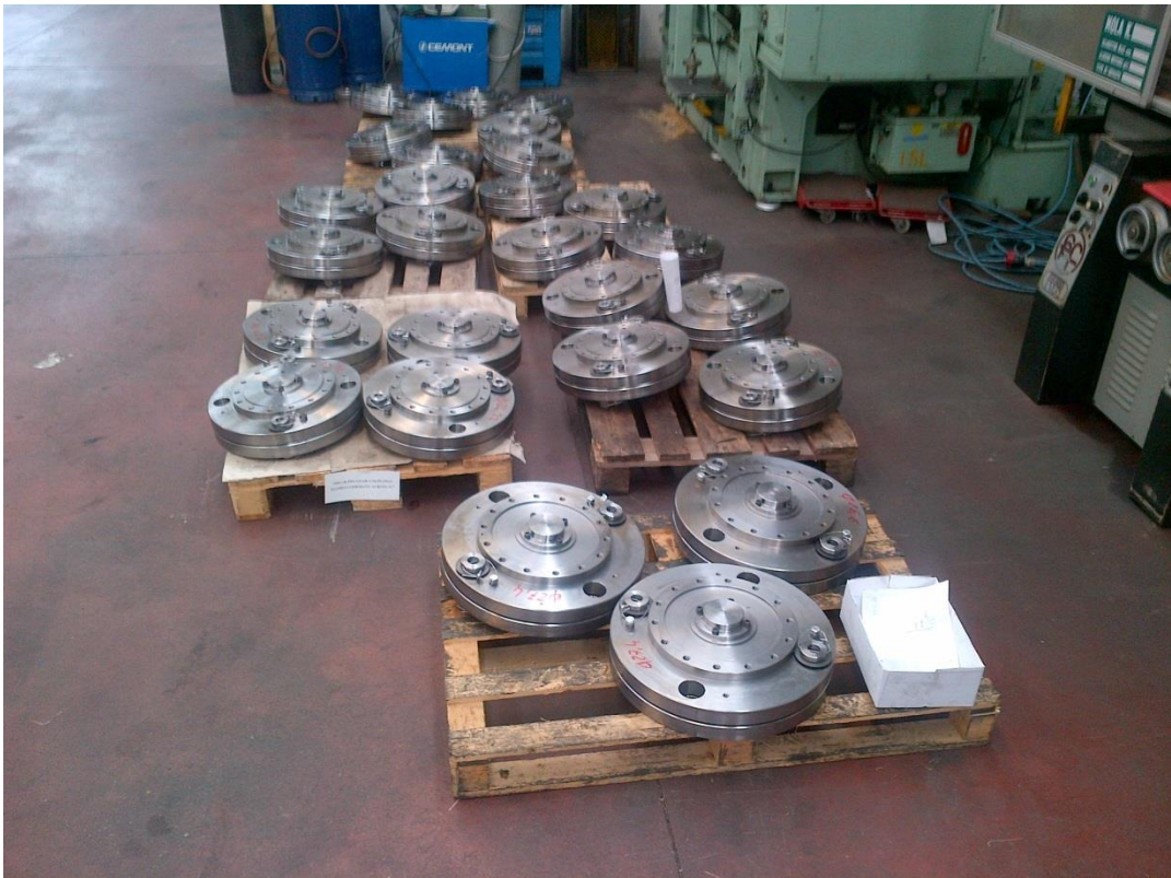
FIG. 19 INTERMEDIATE FLANGES WITH SHEAR PINS SAFETY DEVICE
