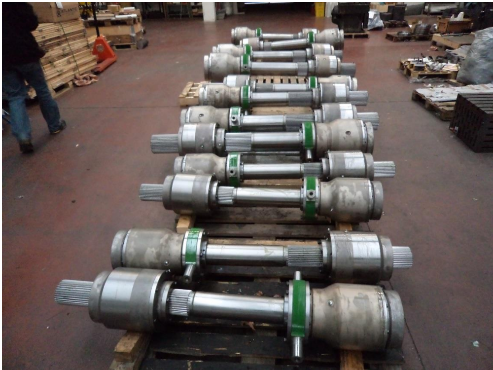
FIG. 52 MILL GEAR SPINDLES FOR BAR MILL
