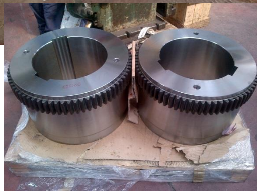
FIG. 39 HEAVY DUTY GEAR HUBS WITH INDUCTION TEMPERING
