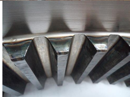
FIG. 40 SLEEVE TEETH WITH INDUCTION TEMPERING
