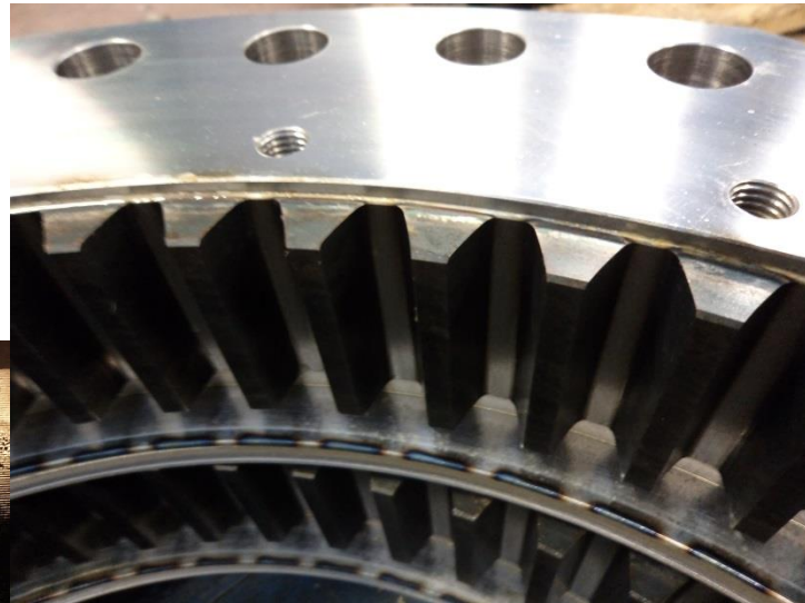
FIG. 47 GEAR TEETH WITH INDUCTION TEMPERING
