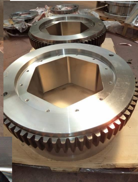
FIG. 41 HEAVY DUTY GEAR HUBS WITH HEXAGONAL BORE AND TEETH WITH INDUCTION TEMPERING
