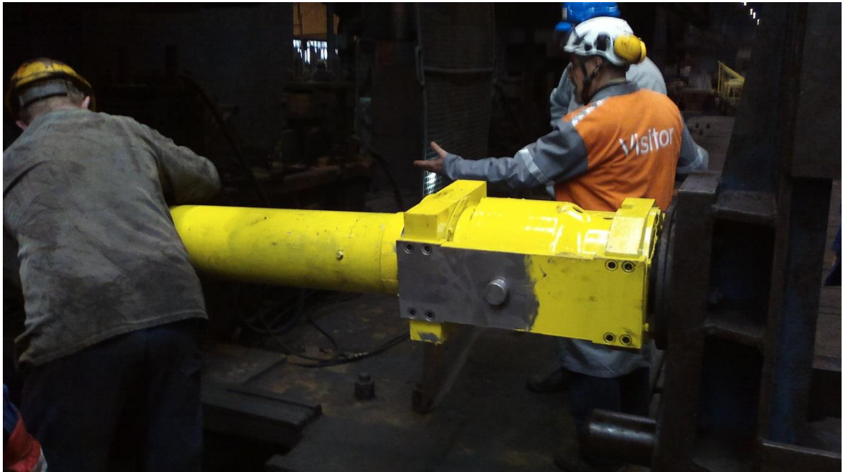
FIG. 58 GEAR SPINDLE ASSEMBLY – COMMISSIONING AT ARCELORMITTAL OSTRAVA – SIEMENS ITALY
