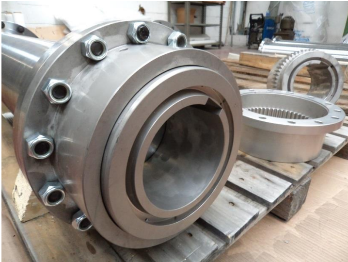
FIG. 14 GEAR COUPLING WITH CONTINUOUS OIL LUBRICATION
