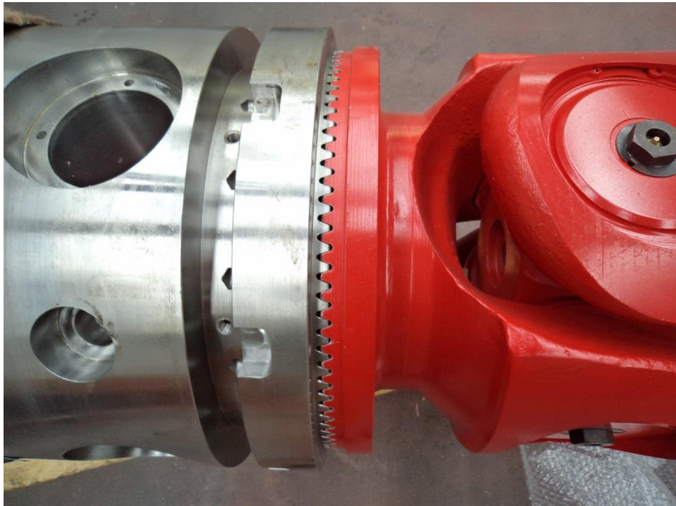
FIG. 69 UNIVERSAL SPINDLE WITH WOBLER – HIRTH SERRATION
