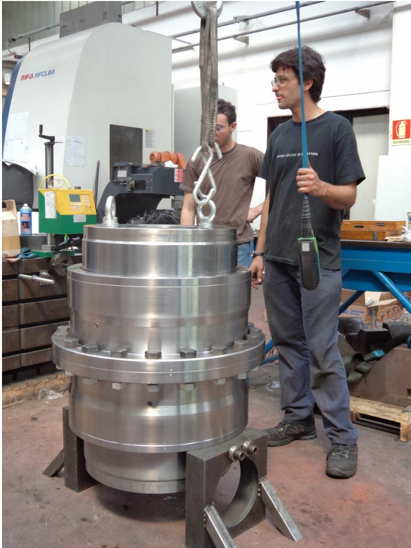
FIG. 28 HEAVY DUTY GEAR COUPLING WITH SEAL COVERS AND LONG HUBS
