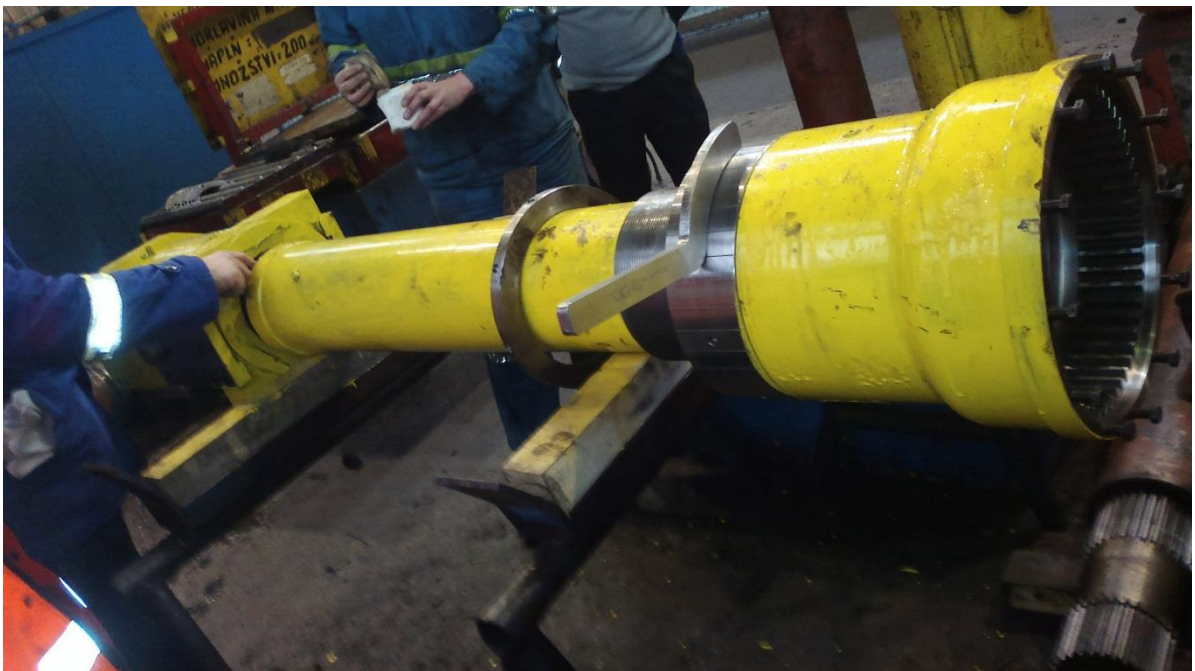
FIG. 59 SPECIAL GEAR SPINDLE ASSEMBLY WITH VARIABLE SET-UP
